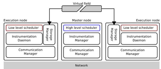
Figure 1: Overview of nodes in the P2G system.
